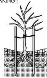
*Proper staking of a bare root tree*
